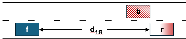
20 21 Figure 2. Graphical description of an incipient passing maneuver wherein 22 the fastest passing vehicle “f” is subjected to potential delay by a 23 micropassing vehicle “b”, thereby a blocking vehicle
