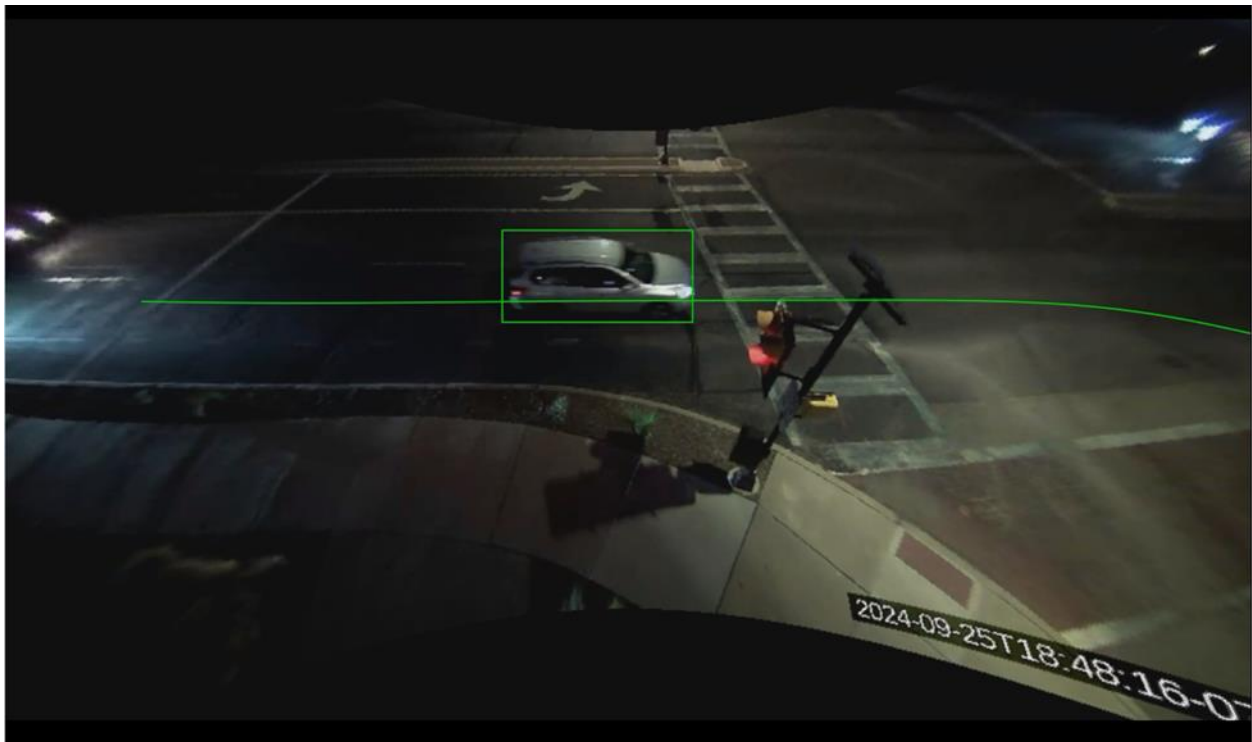
Appendix Photo C7: Drivers pass through the crossing during the FLASHING RED indication after the crossing family has moved to a position not in conflict with the vehicle(s).
