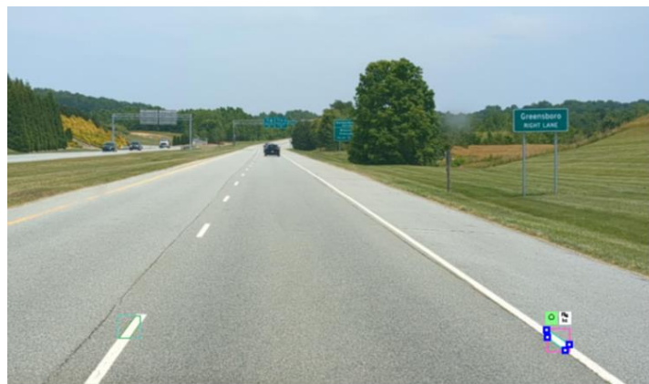
Figure 3. Green Boxed on Lane Line and Edge Line Show Area of Assessment
